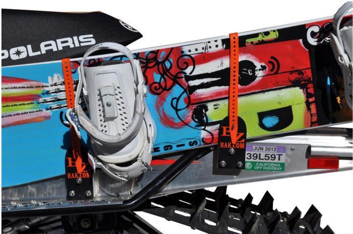
Step 7: Try to place the front rack as low as you can to the side of the tunnel (fig.4). This will increase the angle and raise the back of the board. You can strap the front rack to your board to help free up a hand for next step.
