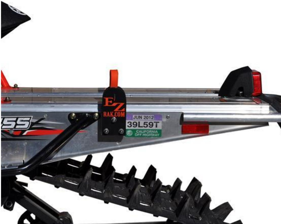
This will help raise the back of the board off the snow. Some snowmobiles have a higher bumper location and you can only use the two bottom holes of the rack for mounting (fig.1B).
